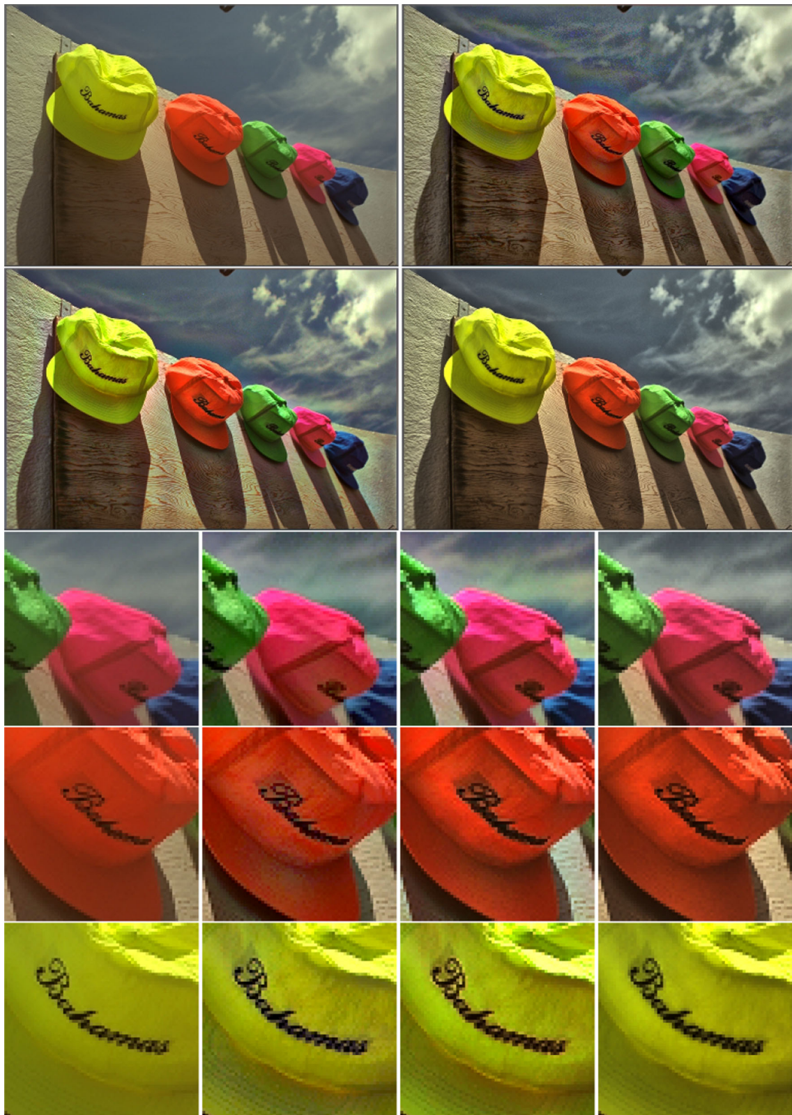
Fig. 8 Contrast enhancement of top left image. Result given by the Euclidean model (29) in the RGB color space (top right) and in the L^*a^*b^* color space (second row, left column). Result given by the model (31) induced by the connection 1-form (58) with the metric (74) encoding the Helmholtz–Kohlrausch effect (73)—last three rows: close-
