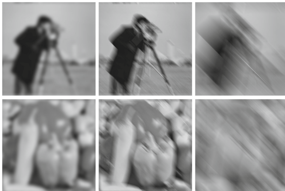
Fig. 2 Degraded images: first row (cameraman) and second row (pepper). From left to right : scenarios of Gaussian blur, medium motion blur and severe motion blur as specified in Table 1
