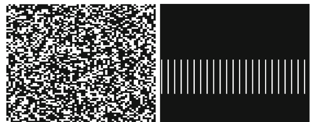
Fig. 15 Missing data pattern. Patterns used in the actress and paper bending sequences, respectively. Each row is a nonrigid frame and each column is a point track. Points in black and in white are marked as visible and occluded, respectively. Left 40 % random missing data. Right 22 % structured missing data
