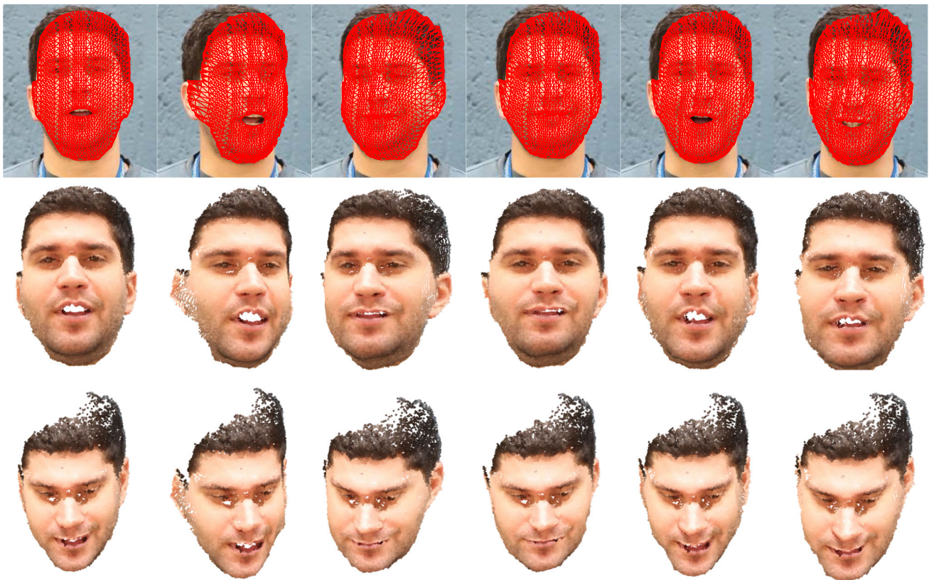
Fig. 17 Niko's sequence: dense 3D point cloud estimation. Top Selected frames #17, #43, #55, #75, #100, and #121 with 3D projected mesh. We display the mesh we use to obtain the mode shape basis. Middle Textured original viewpoint. Bottom Textured general view
