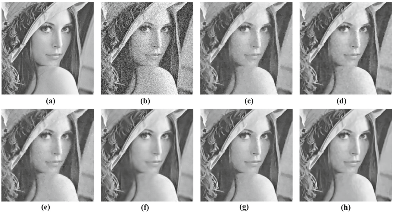
Fig. 6 a Noise-free. b Noisy, PSNR = 18.6. c TV, PSNR = 27.2. d EED, PSNR = 27.9. e TGV, PSNR = 27.4. f NL means, PSNR = 28.4. g New method, PSNR = 28.4. h B3MD, PSNR = 29.2
