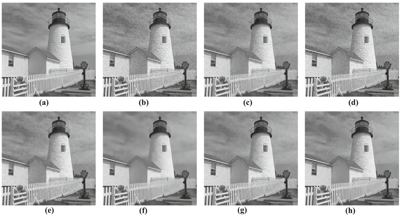
Fig. 8 a Noise-free. b Noisy, PSNR = 18.6. c TV, PSNR = 26.5. d EED, PSNR = 26.2. e TGV, PSNR = 26.3. f NL means, PSNR = 28.3. g New method, PSNR = 28.4. h B3MD, PSNR = 29.9
