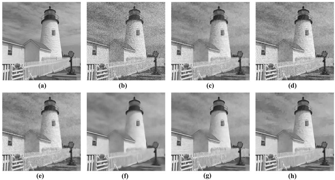
Fig. 9 a Noise-free. b Noisy, PSNR = 14.2. c TV, PSNR = 24.0. d EED, PSNR = 23.7. e TGV, PSNR = 24.0. f NL means, PSNR = 26.1. g New method, PSNR = 25.9. h B3MD, PSNR = 27.4
