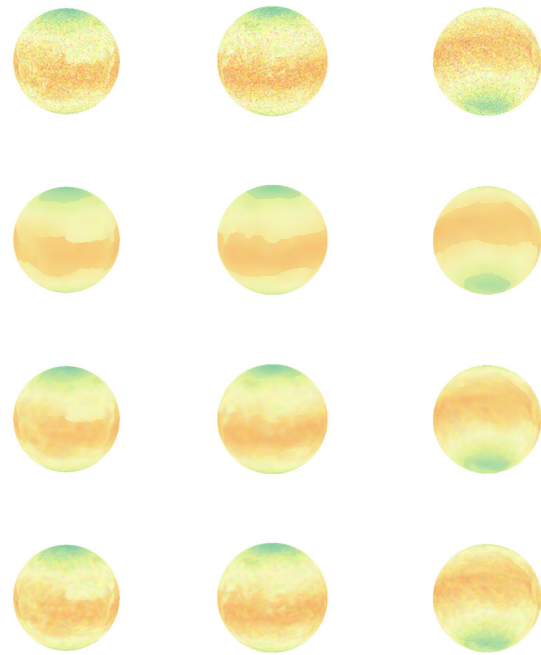
Fig. 13 Denoising of the net radiation data (image with added noise). First row noise-added image to be smoothed. Second row smoothing result using \lambda = 100 . Third row \lambda = 1000 . Fourth row \lambda = 10,000 . First–third columns different viewing angles. The original image is from the NASA Earth Observation data set, [25]
