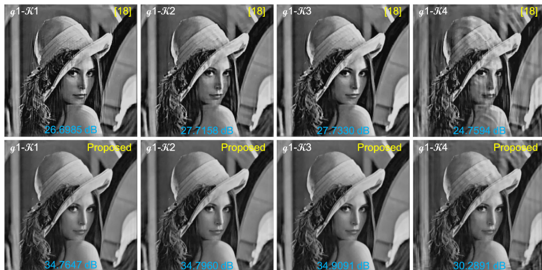
Fig. 9 Deblurred images using the blur-kernels estimated by [29] ( top row ) and the proposed kernel estimation method ( bottom row ) for the multiple-blurred observations simulated from Lena (L) and g_1 = \{\mathcal{K}1 \dots \mathcal{K}4\}
