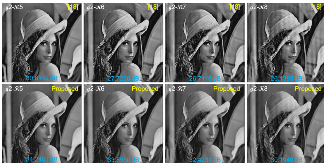
Fig. 10 Deblurred images using the blur-kernels estimated by [29] ( top row ) and the proposed kernel estimation method ( bottom row ) for the multiple-blurred observations simulated from Lena (L) and g2 = \{K5 \dots K8\}
