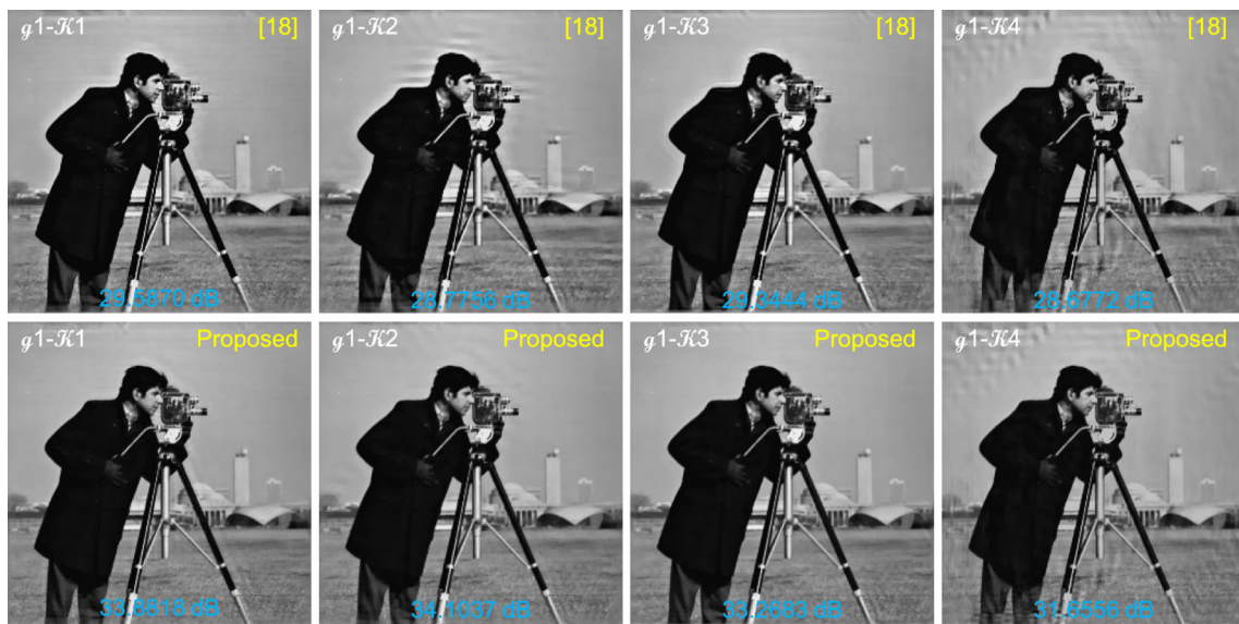
Fig. 7 Deblurred images using the blur-kernels estimated by [29] ( top row ) and the proposed kernel estimation method ( bottom row ) for the multiple-blurred observations simulated from Cameraman (C) and g1 = \{\mathcal{K}1 \dots \mathcal{K}4\} . The figure in each image is the calculated PSNR score
