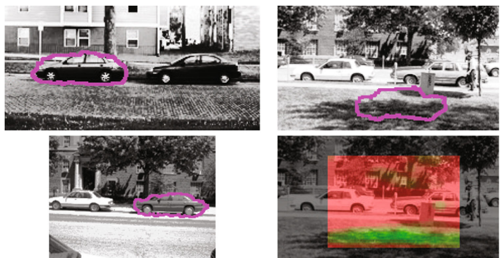
Fig. 14 Locating cars with a spatially inhomogeneous appearance model. Left column . Two successful examples of locating a car within the test image. Right column. Top : A failed example. Bottom : plot of the matching cost depending on translation. Apparently the chosen features are too simple: the shady patch of lawn in the foreground has by far the best cost. Note however that on the right car there is a distinct local minimum (Color figure online)
