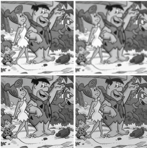
Fig. 9 Experiment 2: Top line degraded image (NL=0.01). Bottom line MNP restorations. Left column blur h_1 ; right column blur h_2
