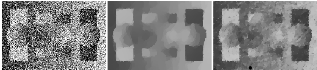
Fig. 4 Justification for the usage of SSIM index. The initial image, seen on Fig. 3, is contaminated with Gaussian noise of variance 0.5 (left). We provide the best SSIM valued (middle) (SSIM = 0.6595, PSNR = 14.02) and the best PSNR valued (right) (SSIM = 0.4955,
