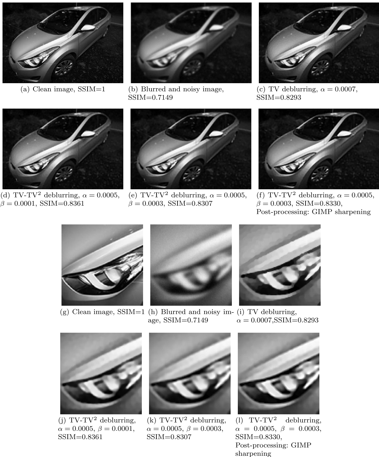
Fig. 13 Deblurring of a blurred (Gaussian kernel of variance \sigma = 2 ) and noisy (additive Gaussian noise, variance 10^{-4} ) natural image. We chose \lambda_1 = 100\alpha , \lambda_2 = 100\beta for these implementations
