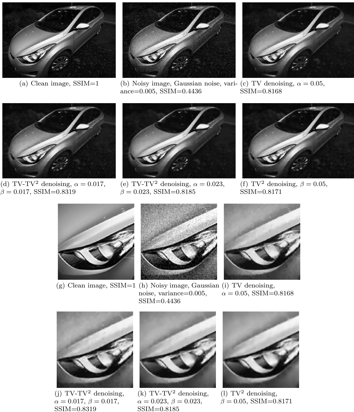
Fig. 10 Denoising of a natural image that has been corrupted with Gaussian noise of variance 0.005. We chose \lambda_1 = \lambda_2 = 1 for these implementations
