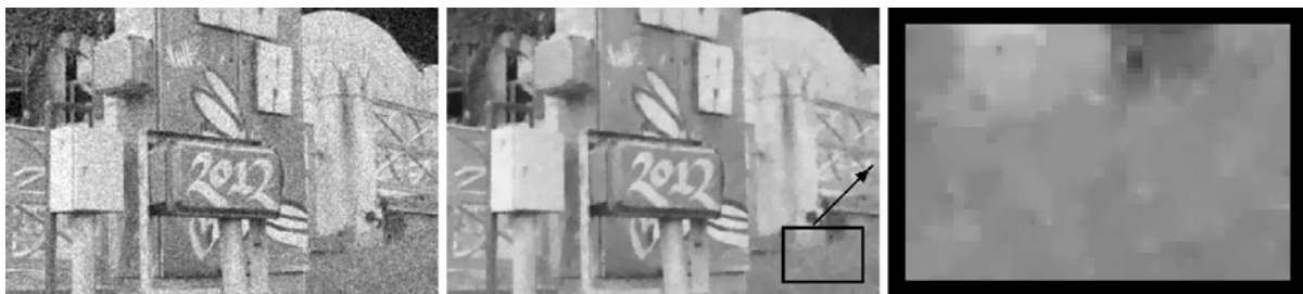
Fig. 2 Total variation image denoising and the staircasing effect: (left) noisy image, (middle) denoised image, (right) detail of the bottom right hand corner of the denoised image to visualise the staircasing effect (the creation of blocky-like patterns due to the total variation regulariser)
