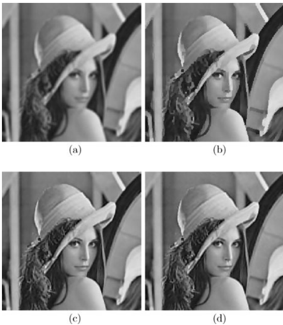
Fig. 9 (a) Image Lena blurred by mask M_1 ; (b) reconstruction using first order finite difference operators; (c) reconstruction using second order finite difference operators; (d) reconstruction using third order finite difference operators
