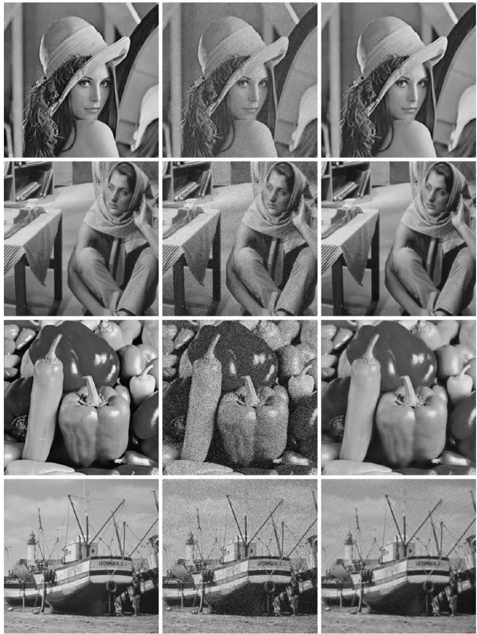
Fig. 7 From left to right: Original, noisy and recovered test images using ANL-means . From top to bottom: Lena corrupted with Gaussian noise with standard deviation \sigma = 25 , Barbara ( \sigma = 20 ), Peppers ( \sigma = 50 ) and Boats with ( \sigma = 55 )
