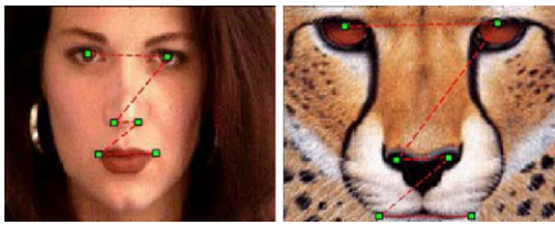
Fig. 2 Six perceptually similar point correspondence are manually marked in the source image (left) and the target image (right). The dotted line shows the order of clicking the feature points
