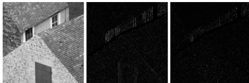
Fig. 15 Image absolute difference between the estimated disparities and the ground truth for a piece of the first pair in Fig. 14. From left to right: piece of image compared in this figure, classical and adaptive SSD errors. Structured errors are observed in smooth parts of the
