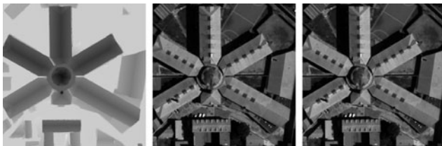
Fig. 7 Synthetic image pair. Left : the disparity ground truth. The background has uniform disparity while the building has a sloped roof. Center and right : image pair
