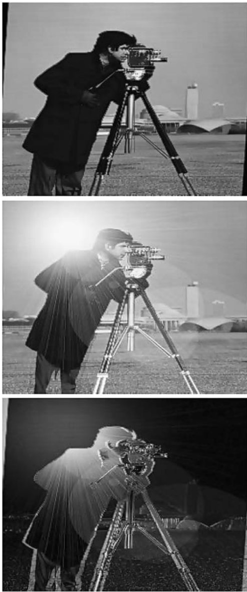
Fig. 4 Lower bound image ( upper ), upper bound image ( middle ) and difference image ( lower ) of the dilated interval-valued camera image
