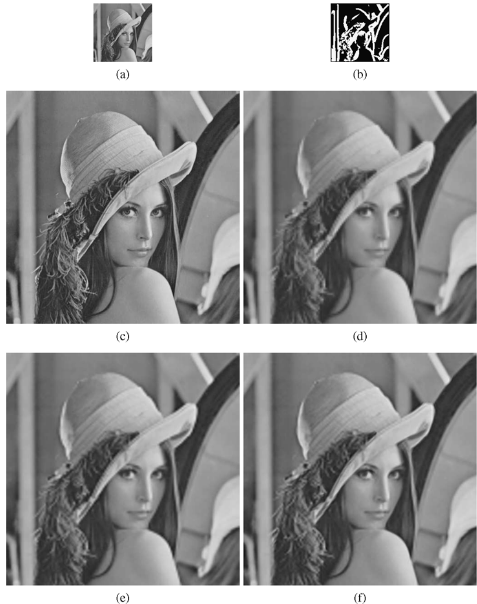
Fig. 6 Enlargement \times 4 of Lena image, \bar{\tau} = 0.0125 : (a) 128 \times 128 initial image (b) coherence map (c) 512 \times 512 original U_0 image (d) bilinear interpolation (e) bicubic interpolation (f) ARBF interpolation
