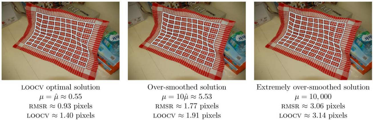
Fig. 4 The visualization grid predicted by the warp for (left) the LOOCV optimal solution parameter, (middle) an exaggerated smoothing parameter and (right) an extreme smoothing parameter corresponding to the asymptotically affine behavior of the warp
