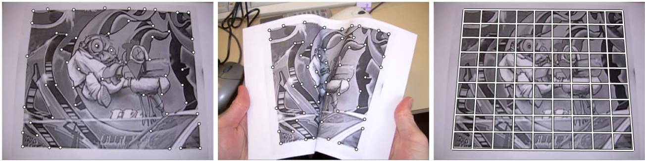
Fig. 5 (left, middle) The source and target images of the self-occluding paper sheet dataset overlaid with the 53 manually clicked point correspondences. (right) The warp visualization grid covering the region of interest
