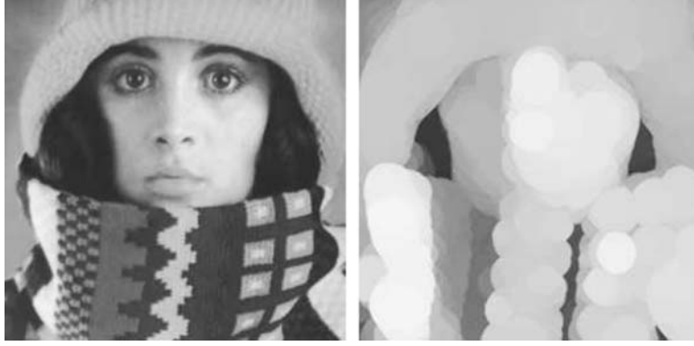
Figure 5. (a) Left: Initial image, 256 \times 256 pixels. (b) Right: Dilation computed by our new FCT scheme ( \Delta x = \Delta y = 1 , \Delta t = 0.5 , 30 iterations).
