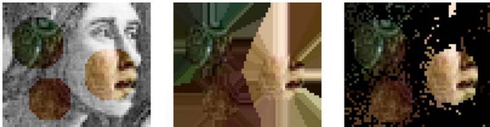
Figure 5. The color of the pixel is extended in the direction of the corresponding Voronoi patch. The constraint check of the projection onto the sub-manifold up to a threshold allows to keep only the color information which is compatible with the known gray information.
