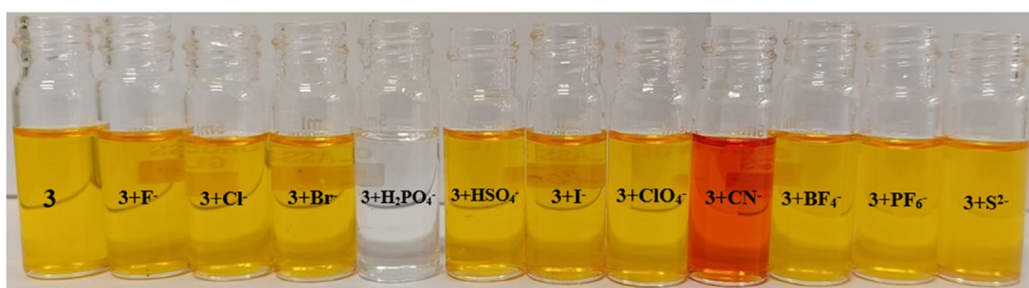
Fig. 5 Colour change in complexes ( 1 \times 10^{-4} M) in the presence of anions ( 3 \times 10^{-4} M) in DMF: a Eu-hqtsc and b Tb-hqtsc
