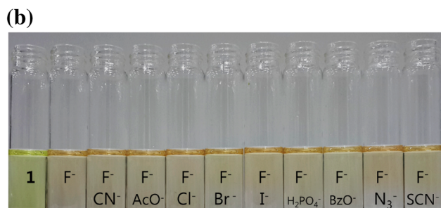
Fig. 5 a Competitive selectivity of 1 (10 \mu\text{M} ) toward \text{F}^- (240 equiv) in the presence of other anions (240 equiv). b The color changes of 1 (10 \mu\text{M} ) in the presence of \text{F}^- (240 equiv) and other anions (240 equiv)
