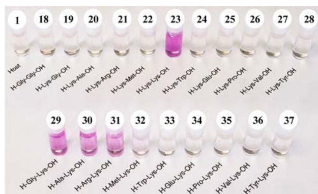
Fig. 13 Visible recognition of the sequence of dipeptides ( 18–37 ) by the host 1 . The concentration of 1 was 1.0 \times 10^{-3} M and those of dipeptides were 1.5 \times 10^{-3} M in the presence of NEP ( 2.5 \times 10^{-2} M) in methanol/water = 10/1. 1 , Host 1 only; 18 , Gly-Gly; 19 , Lys-Gly; 20 , Lys-Ala; 21 , Lys-Arg; 22 , Lys-Met; 23 , Lys-Lys; 24 , Lys-Trp; 25 , Lys-Glu; 26 , Lys-Pro; 27 , Lys-Val; 28 , Lys-Tyr; 29 , Gly-Lys; 30 , Ala-Lys; 31 , Arg-Lys; 32 , Met-Lys; 33 , Trp-Lys; 34 , Glu-Lys; 35 , Pro-Lys; 36 , Val-Lys; 37 , Tyr-Lys
