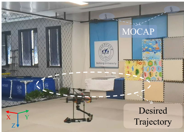
Fig. 9 The scenario of trajectory tracking. The white dashed line indicates the UAV desired trajectory. The MOCAP provides the localization information for the AEROM
