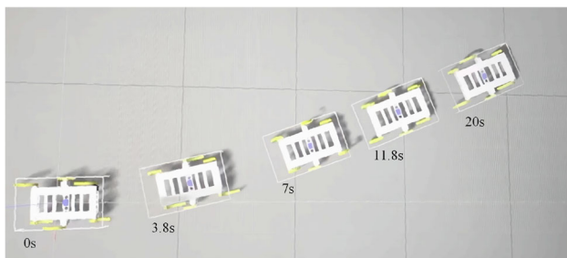
Fig. 13 The directional motion snapshots of BLHR with tripod gaits
