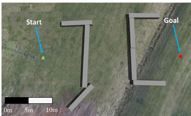
Fig. 24 Demo 7 environment. This environment features two C shaped obstacles one facing the start and one facing the goal.
