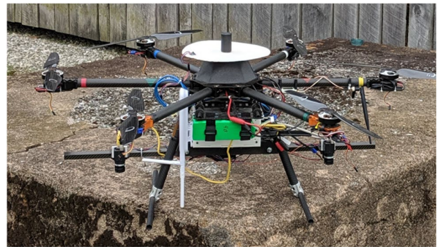
Fig. 3 Tarot T960 hexacopter with custom stereo system and Nvidia TX2
