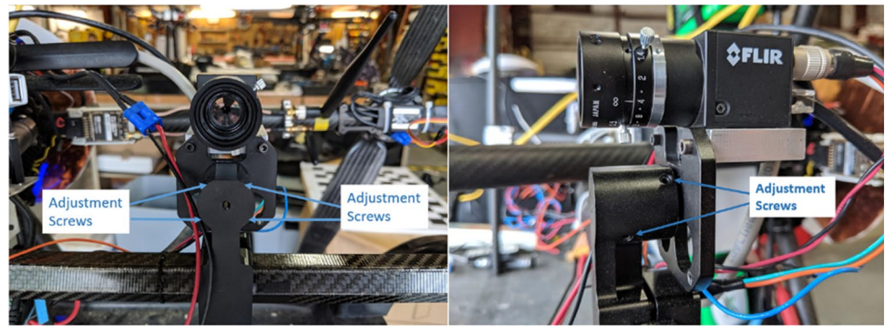
Fig. 5 One of the FLIR/Point-grey cameras mounted on the boom. Mount allows for adjustment which is critical for proper calibration and use
