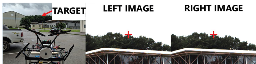
Fig. 6 Example of how the UAV is positioned for calibration and example images showing the alignment process
