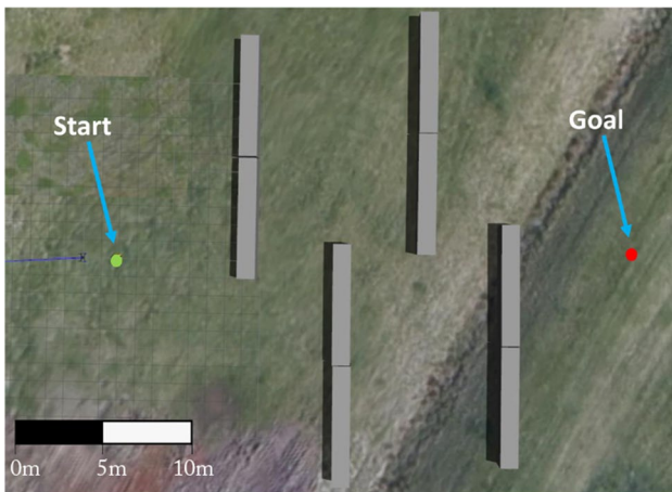
Fig. 23 Demo 2 environment. This environment features long obstacles with a much shorter path through the center. Designed to be a worst case for the RRT explore algorithm
