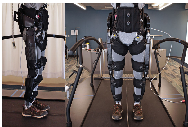
Fig. 7 Experimental setup. The experiment entails walking on a treadmill while being assisted by the Indego Explorer exoskeleton by the hybrid or impedance controller
