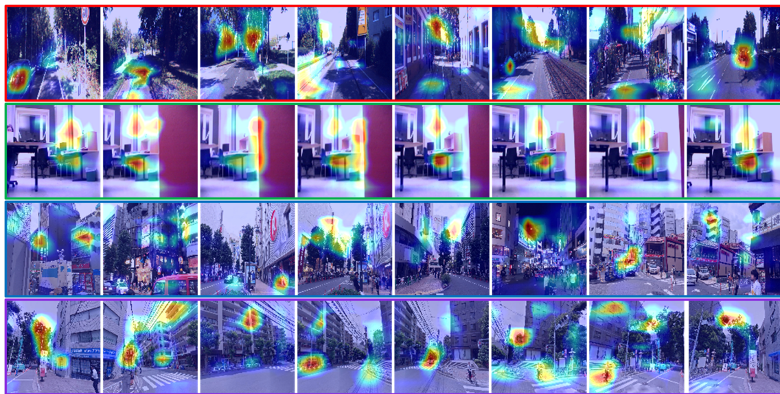
Fig. 6 Some partial images taken from public datasets, from the first row down, the images are taken from KITTI, KTH-IDOL2, TOKYO 24/7 and Tokyo time machine, which presents some salient regions that
