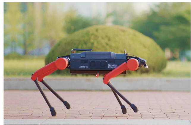
Fig. 1 The proposed whole-body controller, tested on a quadrupedal robot, AiDIN-VI, that has torque sensor at each joint, allows the robot to locomote on various environments
