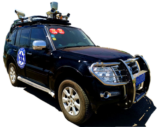
Fig. 9 Our intelligent vehicle used for the experiments. It is equipped with five cameras, a Velodyne HDL-64E S2 LiDAR, and a GPS-aided inertial navigation system
