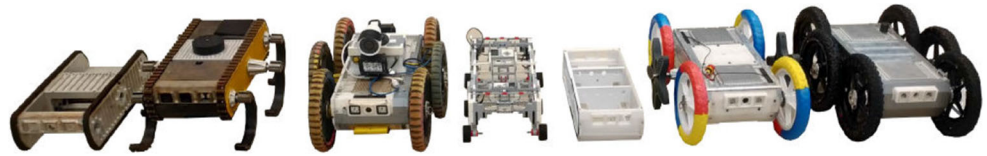
Fig. 3 EspeleoRobô's evolution, from left to right, starting at the first version in 2015 and ending at the current waterproof version of the platform
