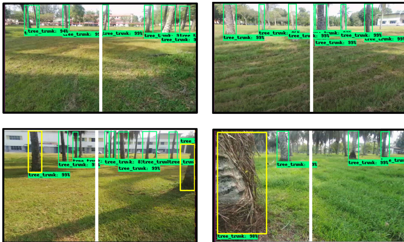
Fig. 10 Examples of safe condition that the UAV is allowed to move forward. The white line represents the direction of the optimum heading and remains in the center of the image as there is no critical obstacle ahead and the UAV is safe to continue its forward motion
