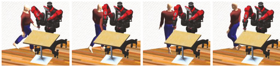
Fig. 9 Simulation of 3-D collision-free motion for picking & placing use-case by right arm. The right arm is in the untucked position before the movement. There is a human model walking in the working
