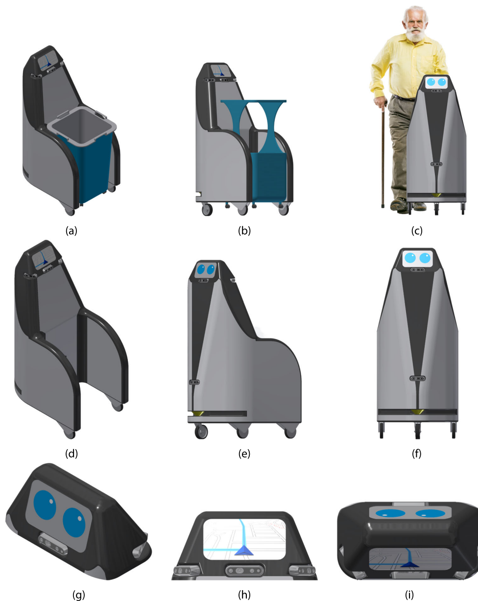
Fig. 5 Visualization of the final design. a and b show different modules for the logistic and drink serving use cases and c illustrates the robot being applied to the guidance use case (background: stock image
