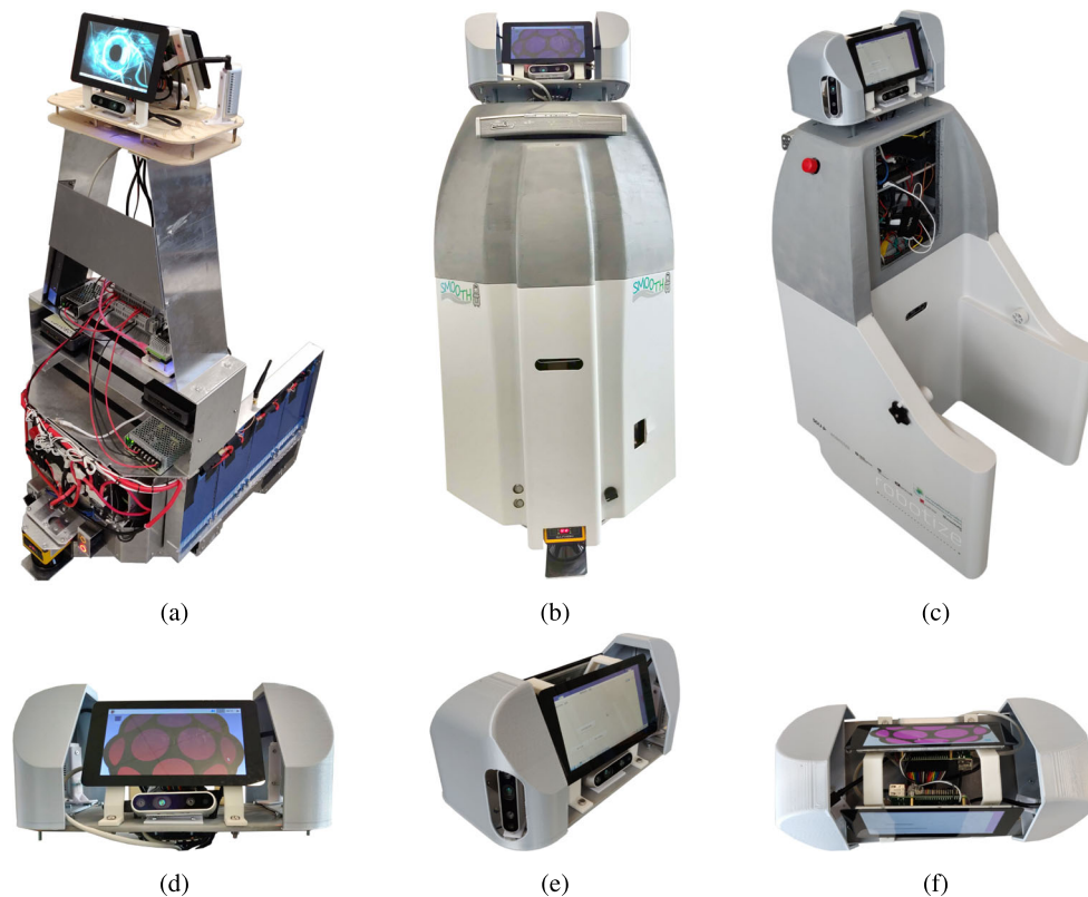
Fig. 12 First prototype of the SMOOTH robot. a shows the robot with all its electronics exposed. b and c shows front and back views of the robot complete with covers and everything installed. d–f shows close-ups of the sensor head
