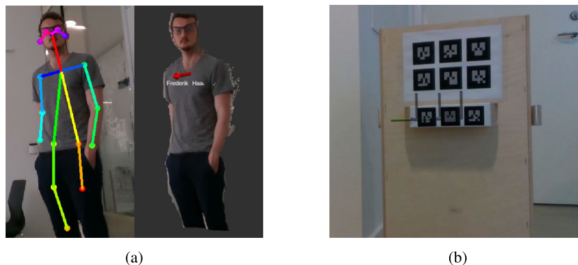
Fig. 7 Example of different sensor processing modules. a Human detector based on OpenPose [7]. It uses the detected keypoints to crop the person pointcloud, estimate torso direction, and recognize the face. b AR marker detection on bin module mockup using the ar_track_alvar ROS package [2]
