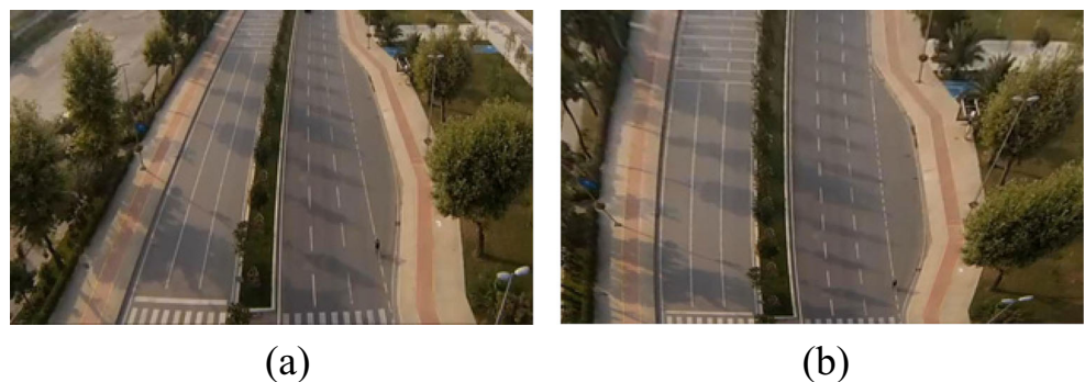
Fig. 3 Road image appearance for a the image plane; b the world plane
