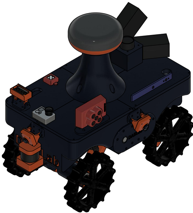
Fig. 4 CAD drawing of the ultra-compact 3D printed robot with a suite of sensors
