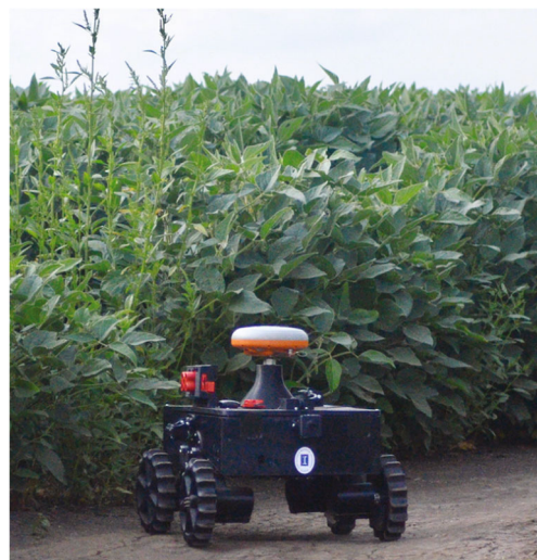
Fig. 3 The mobile robot, termed TerraSentia in off-road terrain
