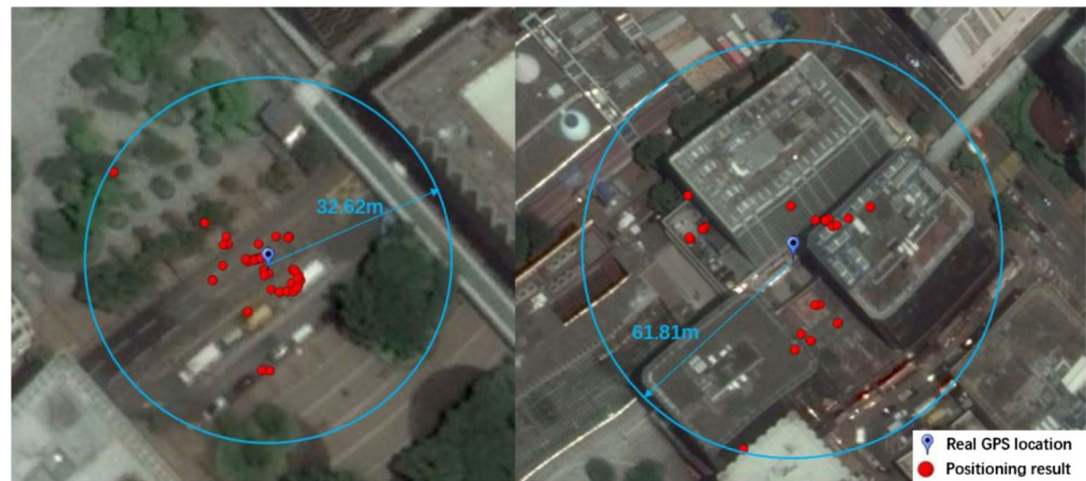
Fig. 10 Experimental GPS positioning result for 30 minutes. The left and right panels show the results in the intersection and the narrow canyon, respectively. Red spots show the positioning result, and the blue balloon shows the real GPS location
