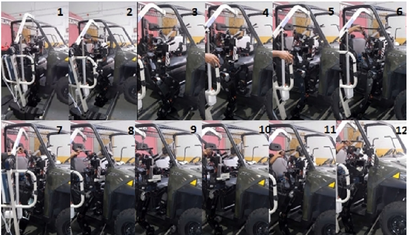
Fig. 32 DRC-Hubo's Step up motion with Polaris (1st half phase)
