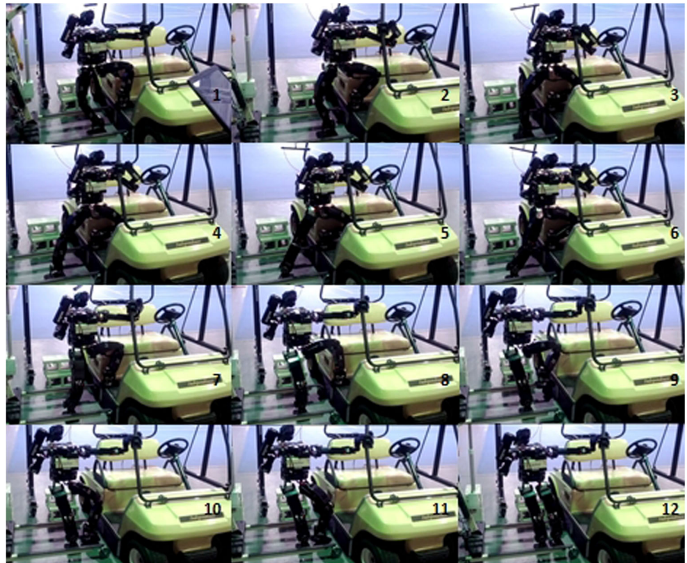
Fig. 27 DRC-Hubo’s Step down motion during egress (2nd half phase)
