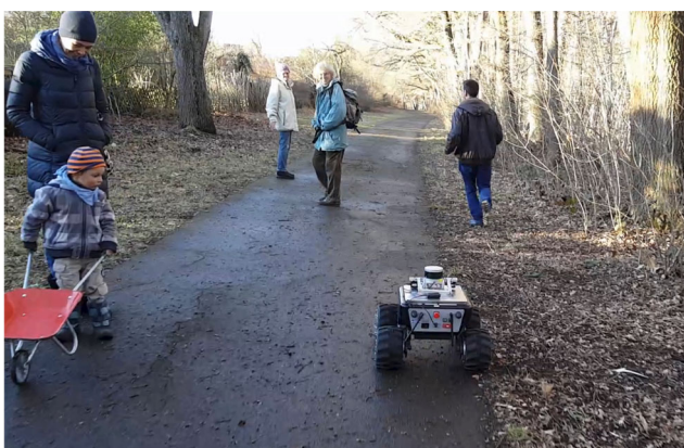
Fig. 20 The robot’s task is to accompany a person at higher speeds in outdoor environments. High level control is needed due to unknown environments and obstacles
