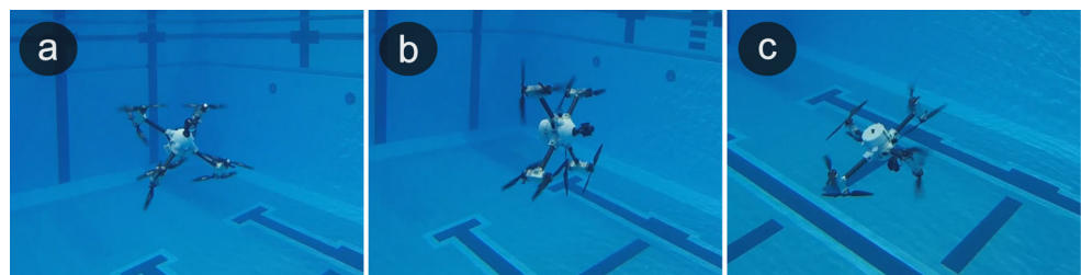
Fig. 1 Experimental platform “Naviator” performing a flip maneuver underwater, shown approaching a forward pitch of 45° in (a), 90° in (b) and 180° in (c)
