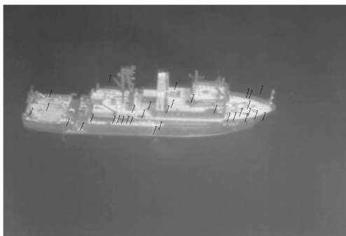
Fig. 6 Optical flow vectors acquired by SIFT on an image captured at the flight experiment
