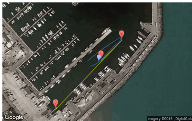
Fig. 15 Trajectory of the ASV during tracking. Point 1,2,3 mark the position of the target at different times
