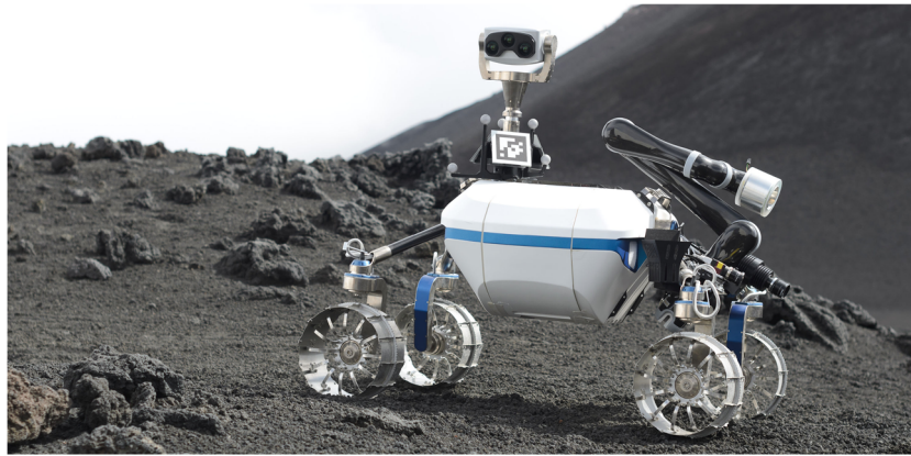
Fig. 32 LRU at lunar analogue test site on Mt. Etna, Sicily, Italy in September 2016
