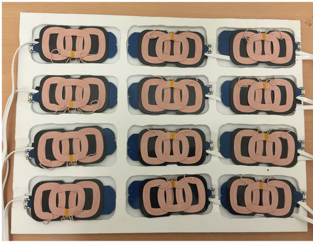
Fig. 5 The utilised prototype charging pad ( 30 \times 40 \text{ cm}^2 ) including 12 independent cells ( M_{4,3} ) supplied with a USB hub (5 V, 1 A)
