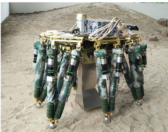
Fig. 1 Robot Octopus III is a robot designed for carrying high payload when traversing uneven terrain. It has unique parallel mechanism legs
