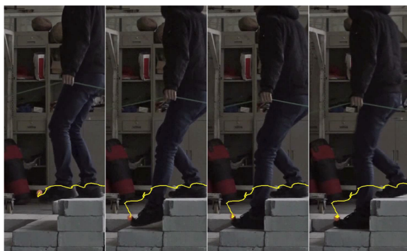
Fig. 12 Foot-tip trajectories during stepping down the obstacle. The step length was short during walking on uneven ground. It is worth noticing that the center of the body did not move out of the supporting foot until the swing foot had actually stepped on the stable ground, which implies that the volunteer was using a static gait while there was no vision system to help him to plan the next step
