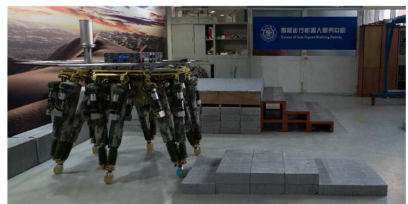
Fig. 18 Experiment settings. The uneven ground is constructed with two layers of the bricks, which is not as high as the obstacle in the human blind walking experiment. This is because the workspace of the leg mechanism is smaller than the serial limb of the human. The max displacement of the prismatic joint is 0.3m, while the height of the brick pile is 0.2m. Moreover, the pile of bricks is placed on the right side of the walking direction, which makes the obstacle not symmetric about the sagittal plane
