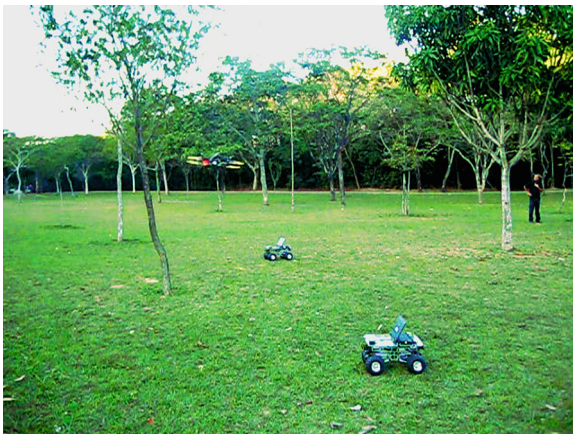
Fig. 1 Real experiment of cooperative navigation using the MRPT with a team of heterogeneous (aerial and ground) under-actuated robots
