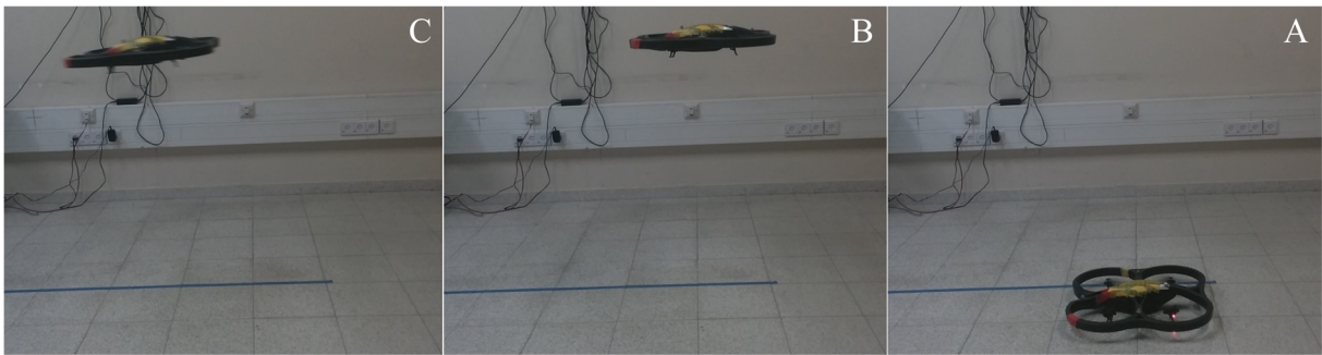
Fig. 11 The AR.drone during forward flight experiment in Ben Gurion University robotics lab. The Optitrack camera system is used to simulate a virtual corridor and data from a simulated image is sent using a wireless interface to the MAV. Lines
