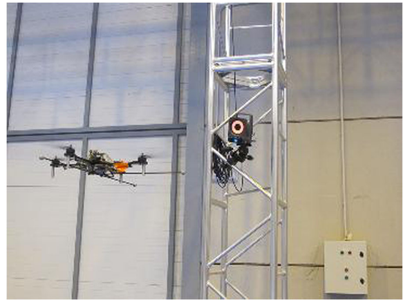
Fig. 7 One of the Hummingbird quadrotors used in the experiments and one of the infrared cameras of the VICON system
