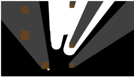
Fig. 8 Top view of occupied areas after occlusions are accounted for. Grey regions are occluded by static obstacles. White areas are areas occupied or occluded according to the system under test. Brown boxes indicate the locations of static obstacles. The sensor is located below the image
