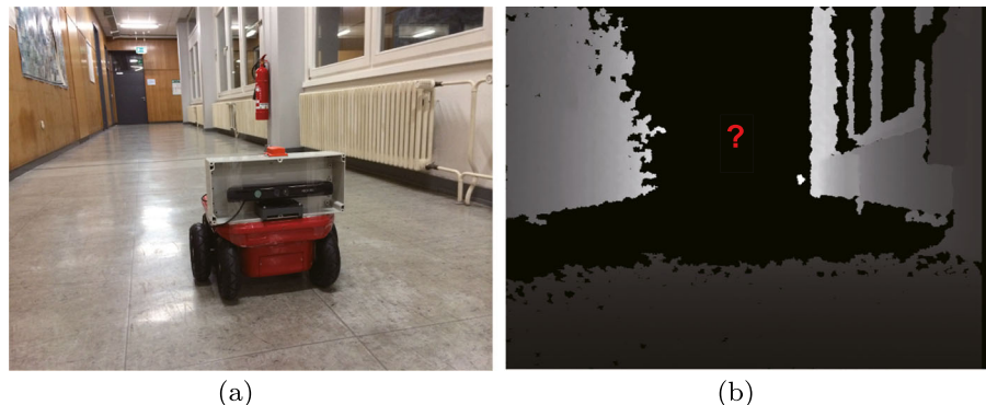
Fig. 1 Kurt2 mobile robot moving through the corridor and the depth image it sensed
