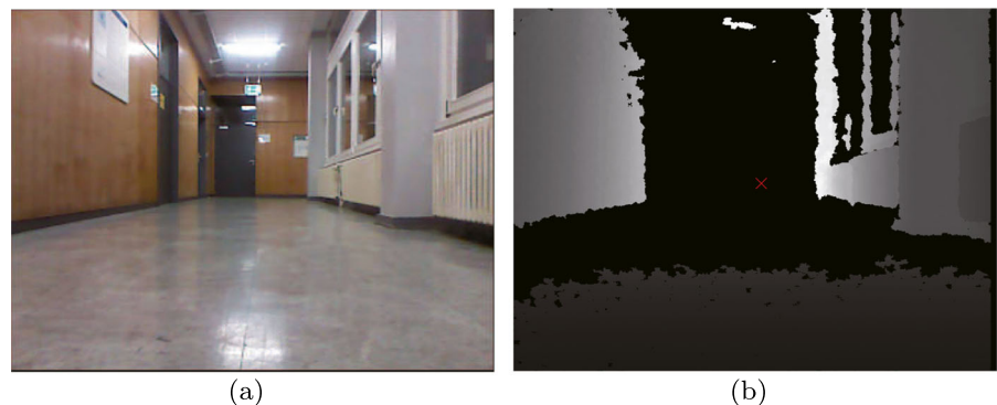
Fig. 4 Vanishing point detection using depth image and multi plane segmentation
