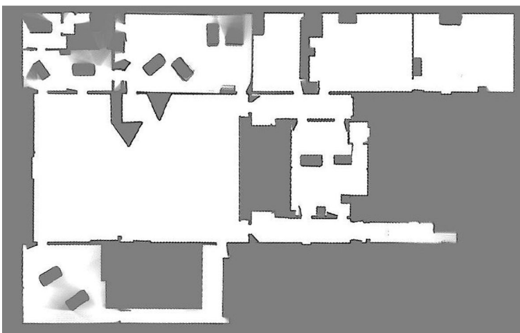
(a) Results by Andrew Howard et al., showing an occupancy grid map, color coded with grayscale for occupancy values between 0 and 1 (image copied from the online Radish dataset repository [21]). The map presented here was obtained using information from all 4 robots.
