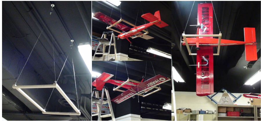
Fig. 13 Moments of inertia testing setup: wire suspended cradle (left); setup to determine the moment of inertia about the pitch axis (top middle), the roll axis (bottom middle), and the yaw axis (right)
